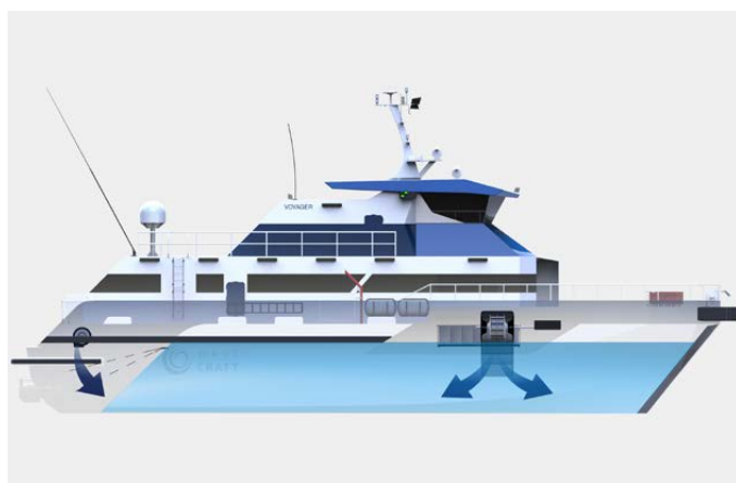
Surface-effect ship (SES) technology
